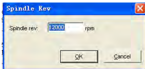
Fig. 4-16 Set spindle rotation speed dialogue box
